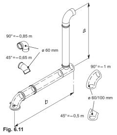
60 mm elbows and extensions can be added to the vertical section.
