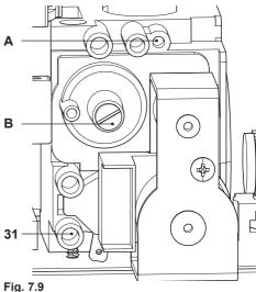
If it does not comply with the required pressure check the gas supply line and governor for faults and/or correct adjustment.
