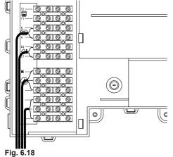
Allow the cables to exit the boiler by using the relevant cable clamps "U" (Fig. 6.19).
