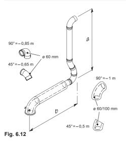
Each additional elbow reduces the overall acceptable length of the flue system as follows:
