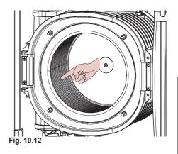
If the condensate primary exchanger elements are dirty (notable only after removing the burner body), brush them using a bristle brush and remove the dirt using a suction device.
